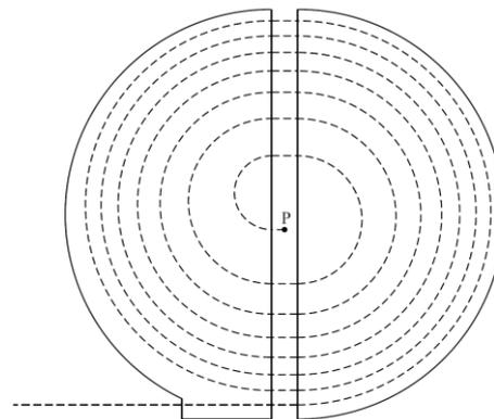
An electric field is located in the space between the two drums. Because the drums are connected to an alternating voltage source, this field keeps changing direction.
