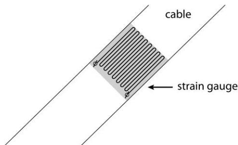
This wire has a resistance of  $350 \Omega$  and a diameter of  $40 \mu\text{m}$ .
