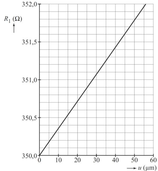
The strain gauge has a length of 6.1 cm and has been glued to a bridge cable of 198 m in length. The diagram of figure 5 shows the relationship between the resistance and the stretching of the strain gauge. If the cable of the bridge stretches 12 cm due to too much traffic, an alarm sounds.
